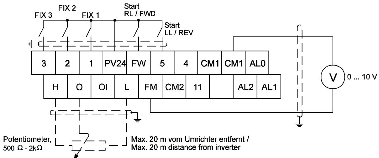
After the above mentioned parameters have been adjusted, the frequency inverter can be started via the input FW in clockwise direction. Input 5 (= REV) will start the equipment in anti-clockwise direction. Closing FW and REV at the same time will cause to stop the inverter.
