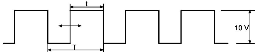
2.) Digital frequency actual value: Supplies a digital frequency signal corresponding to the output frequency
