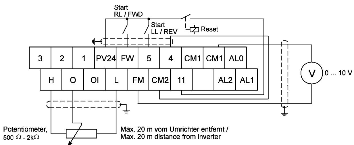
After the above mentioned parameters have been adjusted, the frequency inverter can be started via the input FW in clockwise direction. Input 5 (= REV) will start the equipment in anti-clockwise direction. Closing FW and REV at the same time will cause to stop the inverter.
