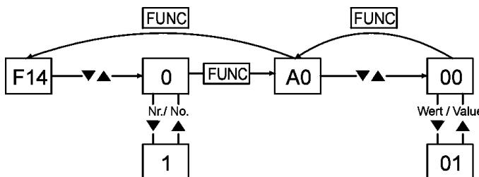
After changing a value make sure to store it by pressing the FUNC key. During operation it is not possible to adjust parameters. They can be only selected and displayed. F14 will always display the last adjusted parameter.
