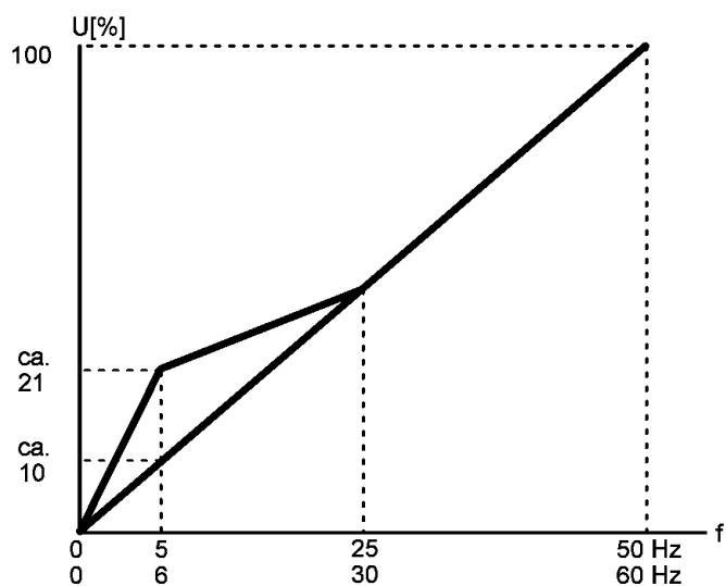
The adjustment only takes effect if V/f control mode is used. In case of Sensorless-Vector-Control (SVC1, SVC2) nothing will happen. In the case of adjustment in real time, press the FUNC key to store the value.
