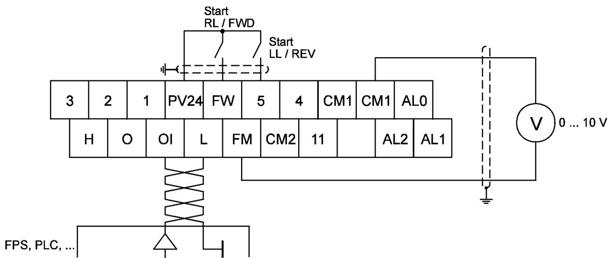
Wiring of the control terminals:
