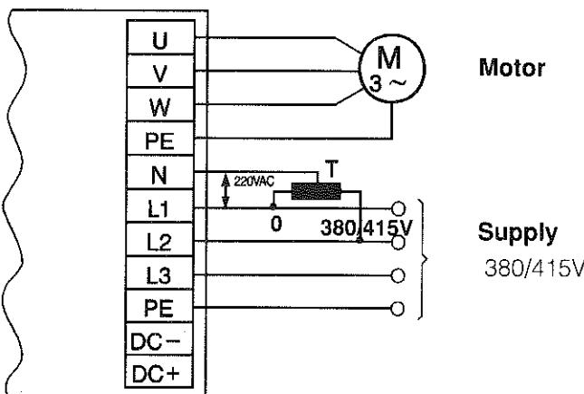
**Note:** Check that the supply to the electronics (between N & L1) is 220/240V before connecting.
