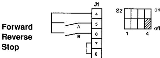
**Stop function:** If A **and** B are both closed **or** open.
