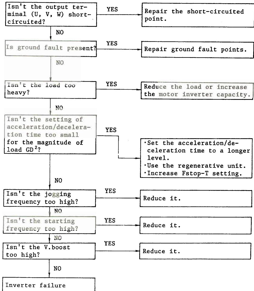
Instantaneous power failure TRIP (Inst. P-F)
