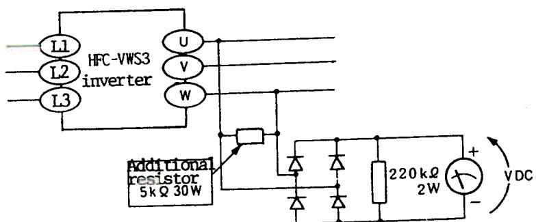
Fig. 22 Output Voltage Measuring Circuit
