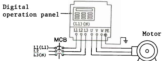
For the standard setting of this inverter, the frequency setting, run and stop are designed to be carried out on the digital operation panel.
