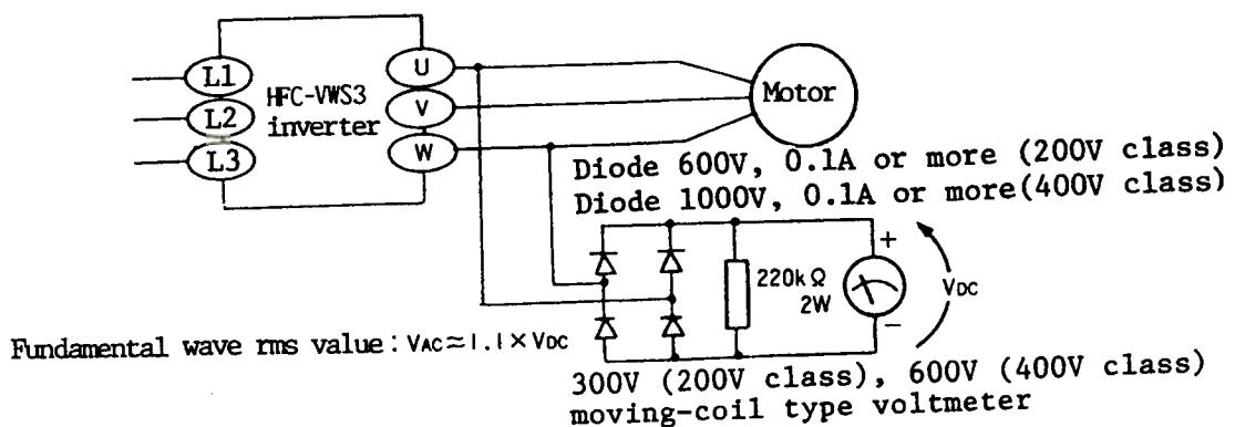
Fig. 21 Output Voltage Measuring Circuit
