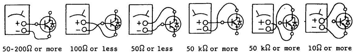
Fig. 25 Inverter Module Acceptability Checking Method
