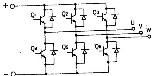
Fig. 23 Circuit Diagram at Inverter Module Unit
