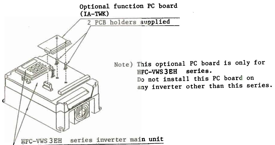
Fig. 19 PC Board (Optional) Installation
