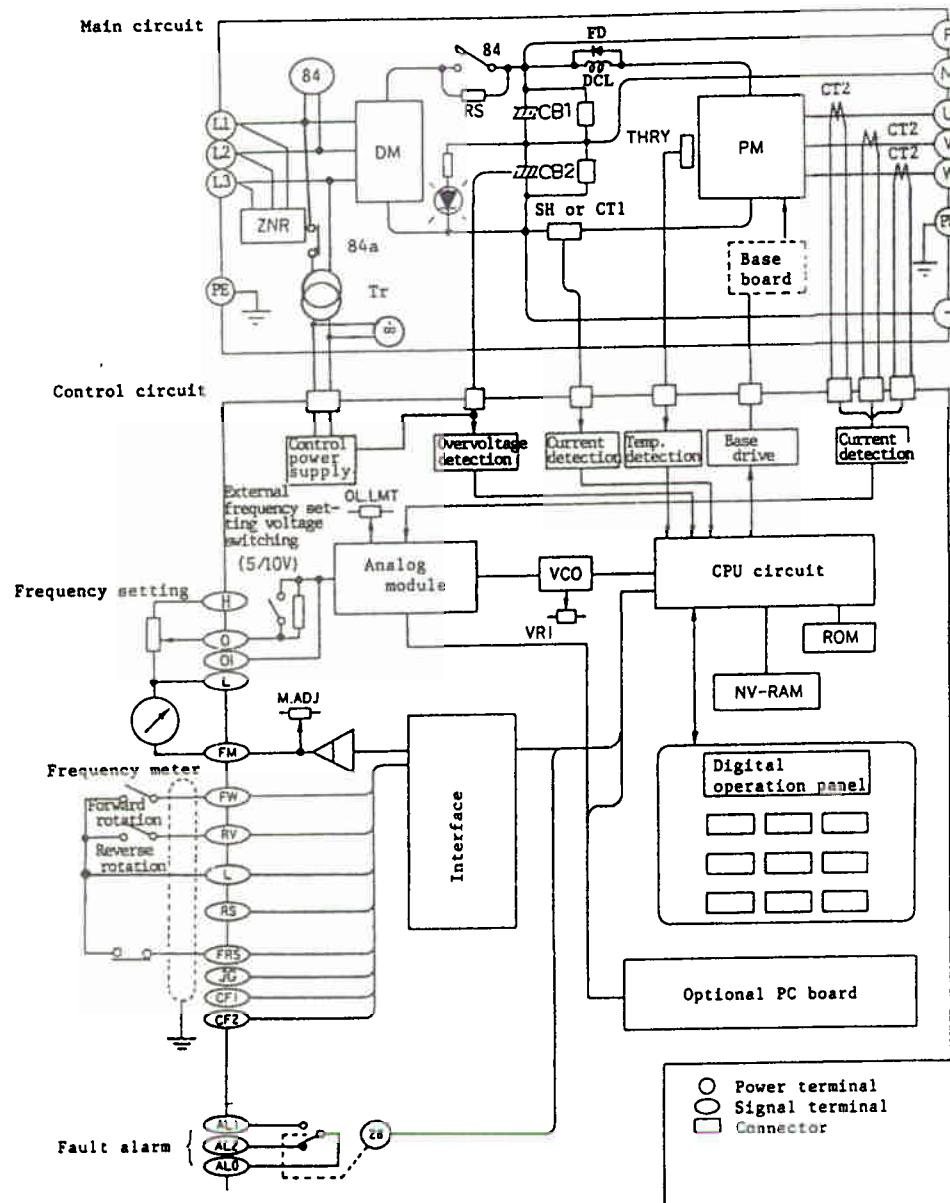
Fig. 4 (b) Circuit Configuration (For 400V Class: 22HF3EH or less)
