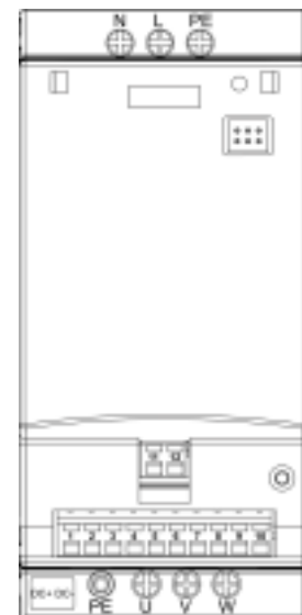
Figure 2-8 MICROMASTER 410 Connection Terminals
